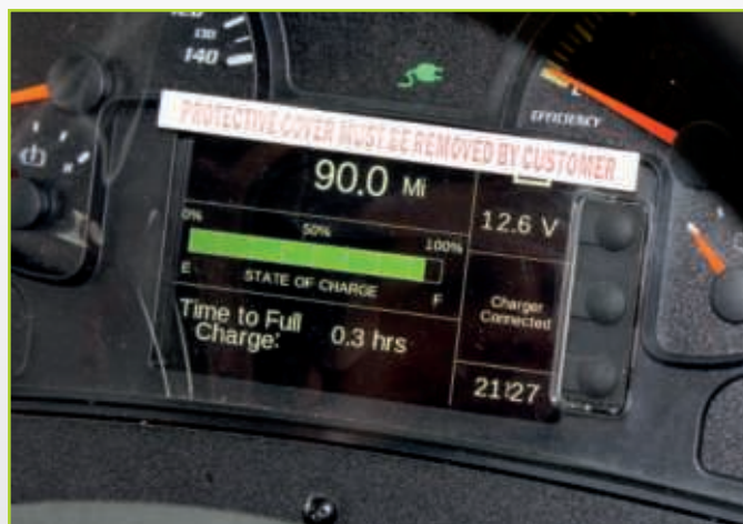
Display shown on screen above steering wheel when charging.
