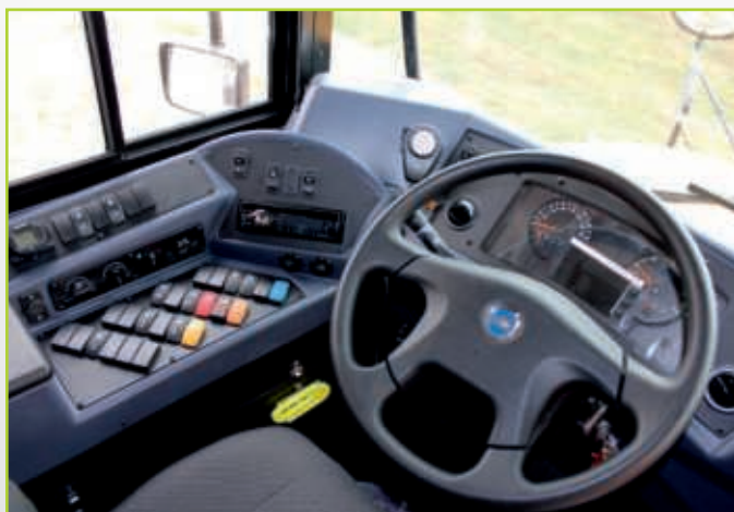
Most of the buses controls are similar to a diesel powered bus, except for the screen above the steering wheel.
