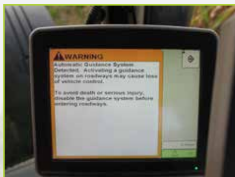
Automatic Guidance Systems warn the operator about roadways, but they do not remind you about other hazards such as power poles.
